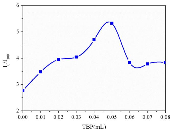
Fig. 3. Quenching ratio ( $I_0/I_{100}$ ) versus the amount of TBP.
