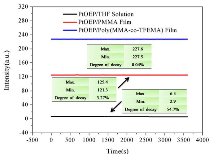
Fig. 6. Photostability of the PtOEP/poly(MMA-co-TFEMA) film, PtOEP/PMMA film, and PtOEP in THF solution.
