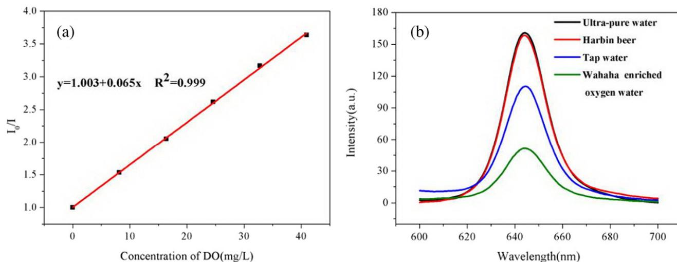
Fig. 7. (a) S-V plot of the sensing film (b) Fluorescence intensity in different water samples.
