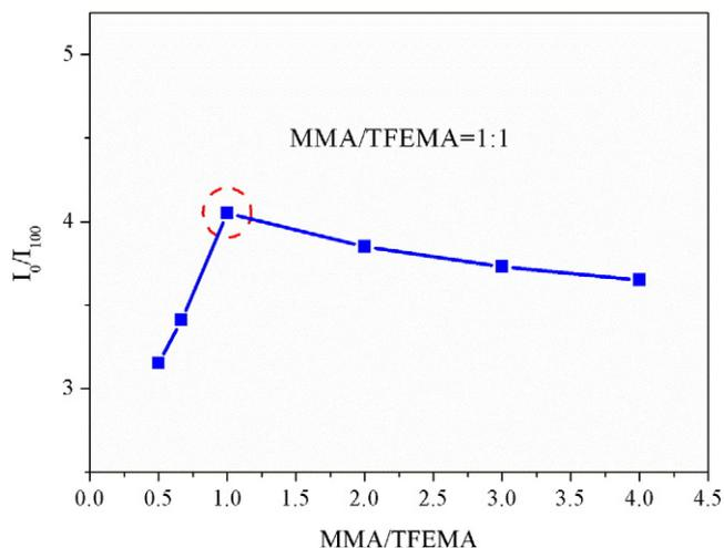
Fig. 2. Quenching ratio ( $I_0/I_{100}$ ) versus monomer ratios (MMA/TFEMA).
