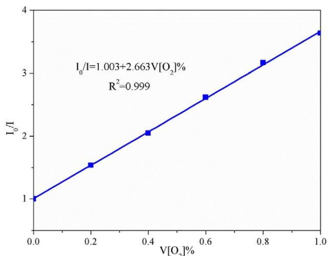
Fig. 5. Stern-Volmer equation of PtOEP/poly(MMA-co-TFEMA) oxygen sensing film.
