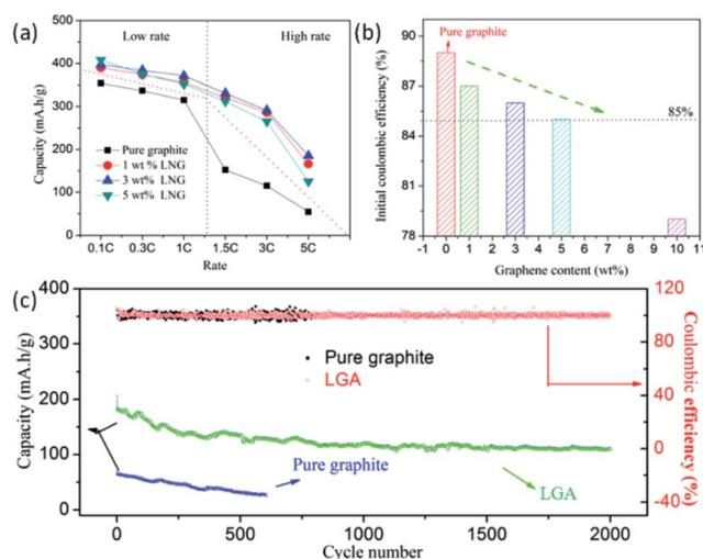
Fig. 5 (a) Discharge rate capability of LGA with 0, 1, 3, and 5% LNG, (b) initial coulombic efficiency of LGA with 0, 1, 3, and 5% LNG, and (c) lithiation/delithiation capacity and coulombic efficiency of LGA electrode cycled at rate of 5C for 2000 cycles.
