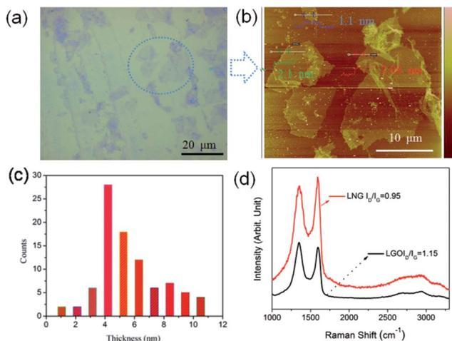
Fig. 2 (a) Optical micrograph of graphene platelets. (b) AFM image of selected graphene sheet. (c) Statistical measurement results of graphene thickness for 80 randomly selected sheets, where thickness ranges from 1 to 10 nm, and (d) Raman spectra (excited by 532 nm laser) of LGO and LNG.
