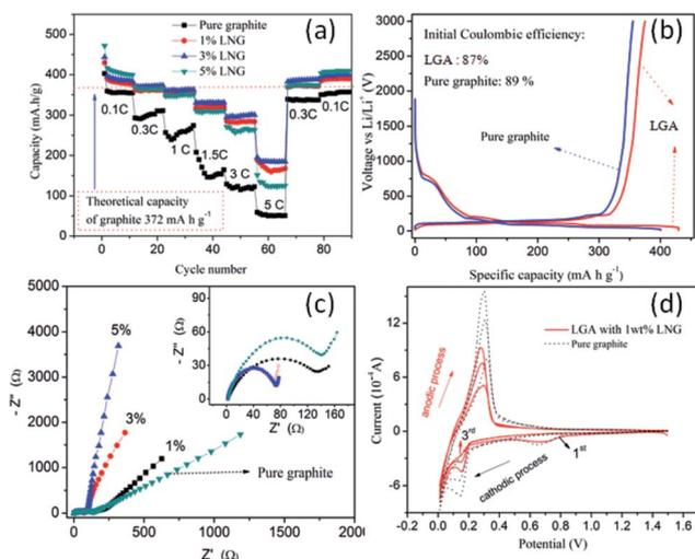
Fig. 4 (a) Rate capability of pure graphite and LGA anode with 1, 3, and 5 wt% (b) charge and discharge curves of LGA anode with 0 and 1% at 0.1C, (c) Nyquist plot of pure graphite and LGA with 1, 3, 5 wt% LNG, showing imaginary part versus real part, and (d) CV curves of the 1<sup>st</sup>, 2<sup>nd</sup>, and 3<sup>rd</sup> cycles of LGA composite with 1 wt% LNG and pure graphite.
