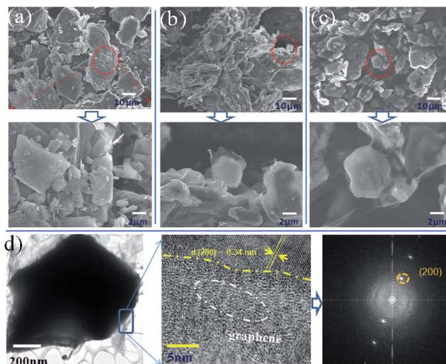
Fig. 3 SEM images of (a) pure graphite and (b, c) LGAs with 1 and 3 wt% LNG, respectively. (d) TEM images of LGA with 1% LNG.
