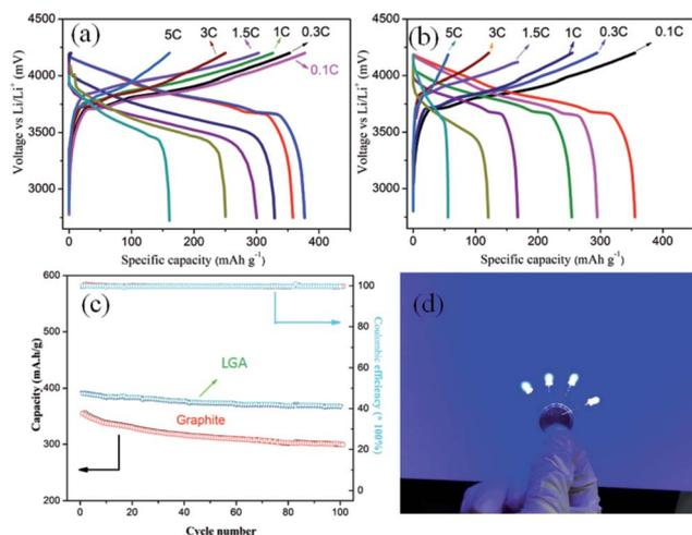
Fig. 6 (a) Voltage profiles of LGA/ $\text{LiCoO}_2$  full cell. (b) Voltage profiles of pure graphite and  $\text{LiCoO}_2$  full cell at a rate of 0.1, 0.3, 1, 1.5, 3, and 5C. (c) Cycling performance of LGA/ $\text{LiCoO}_2$  full cell at 0.1C. (d) Digital photograph of LED powered by LGA/ $\text{LiCoO}_2$  full cell.
