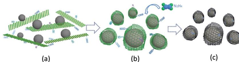
Fig. 1 Illustration of LGA synthesis process: (a) solution containing graphite and LGO, (b) graphite wrapped by LGO, and (c) LGA.
