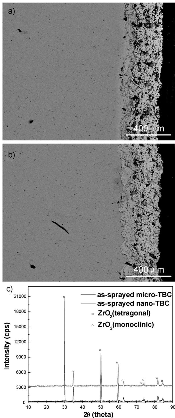
**Figure 1.** SEM cross-sectional micrographs of the as-sprayed coatings: (a) micro-TBC; (b) nano-TBC; (c) XRD patterns of as-sprayed coatings
