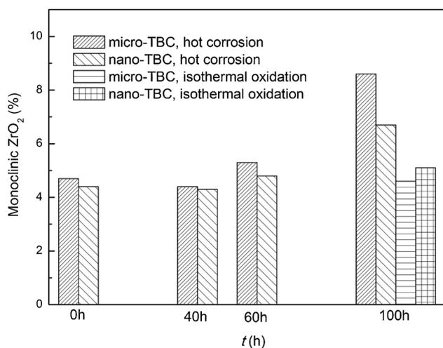
**Figure 5.** Volume fraction of monoclinic phase in the coatings before and after hot corrosion or isothermal oxidation
