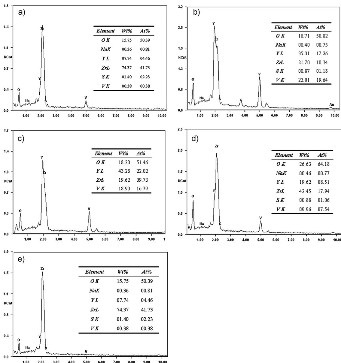
**Figure 3.** EDS spectra from the points on the surface of the coatings in Fig. 2 reveal the corrosion products pointed out by dotted arrow: (a) micro-TBC, after 60 h of corrosion; (b) micro-TBC, after 100 h of corrosion; (c) nano-TBC, after 60 h of corrosion; (d) nano-TBC, after 100 h of corrosion and (e) EDS spectrum from the rectangular area in Fig. 2c
