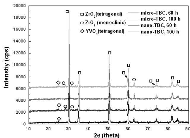
**Figure 4.** XRD patterns show the surface components after hot corrosion
