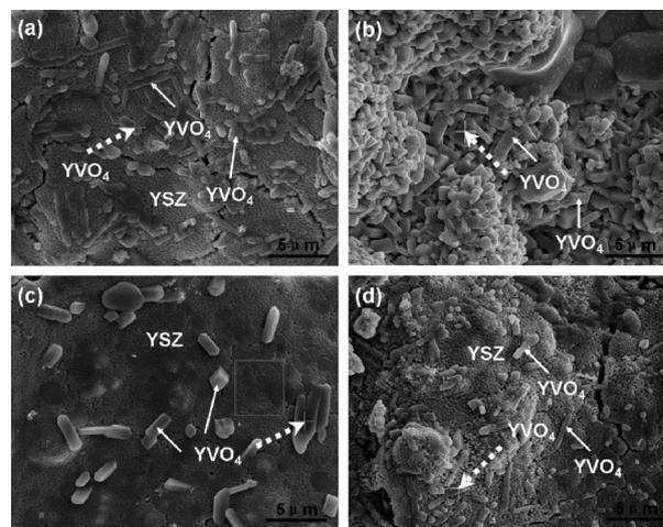
**Figure 2.** SEM micrographs show the surface morphology of coatings after hot corrosion: (a) micro-TBC, after 60 h of corrosion; (b) micro-TBC, after 100 h of corrosion; (c) nano-TBC, after 60 h of corrosion; (d) nano-TBC, after 100 h of corrosion
