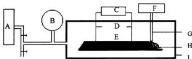
**Figure 1.** Schematic diagram of high pressure SHS chamber (A. oxygen, B. oxygen pressure meter, C. recorder, D. thermocouples, E. the reactants, F. ignitor, G. tungsten wire, H. ignition agent, I. SHS chamber).
