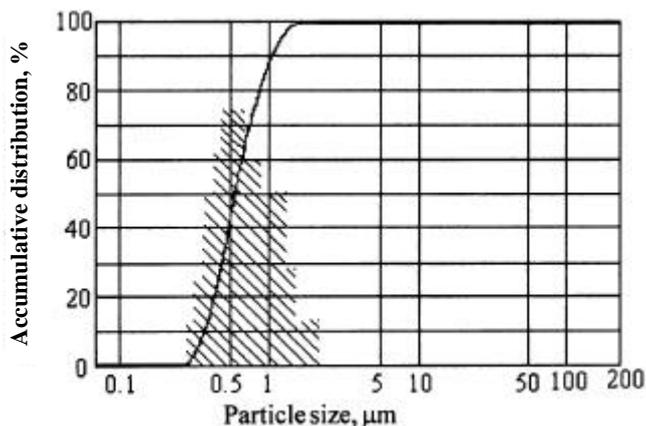
**Figure 4.** Size distribution of Ni-Zn ferrite powders obtained at 1000°C.
