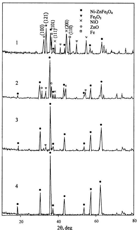
**Figure 5.** The XRD results of the products at different combustion temperatures (1. 700°C; 2. 900°C; 3. 1000°C; 4. 1200°C).
