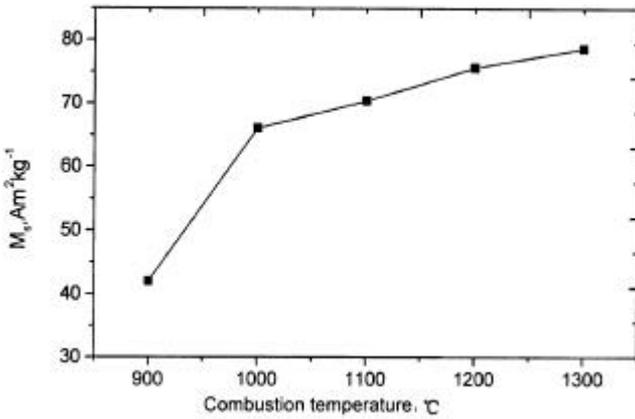
Figure 7. Maximum saturation magnetization,  $M_s$  vs combustion temperature.
