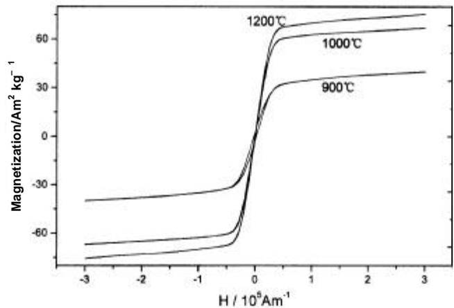
Figure 9. Hysteresis loops for SHS ferrite powders prepared at different combustion temperatures.
