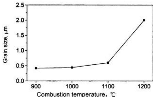
**Figure 3.** The relationship between grain size of Ni-Zn ferrite powders and combustion temperature.
