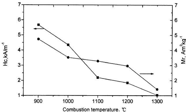
Figure 8. Coercivity force,  $H_c$  and residual magnetization,  $M_r$  vs combustion temperature.
