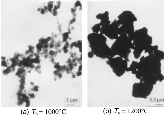
Figure 6. TEM photographs of Ni-Zn ferrite powder.
