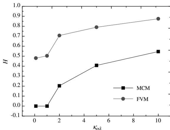
**Fig. 3** *H* values for different absorption coefficients by MCM and FVM in the case of normal laser incidence.
