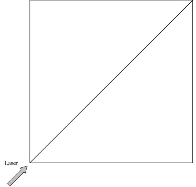
Fig. 2 Physical model of oblique laser incidence on a two-dimensional participating medium.
