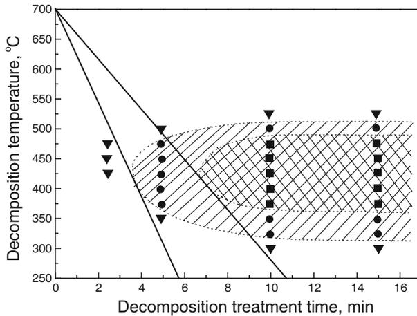
**Fig. 5** Isothermal formation of a magnetite layer at the wüstite-steel interface: *black square* continuous magnetite ( $\text{Fe}_3\text{O}_4$ ) layer, *black circle*  $\text{Fe}_3\text{O}_4$  nucleation, and *inverted triangle* no visible  $\text{Fe}_3\text{O}_4$  was observed [10]
