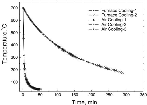
**Fig. 1** Continuous cooling curves from the temperature of 700 °C
