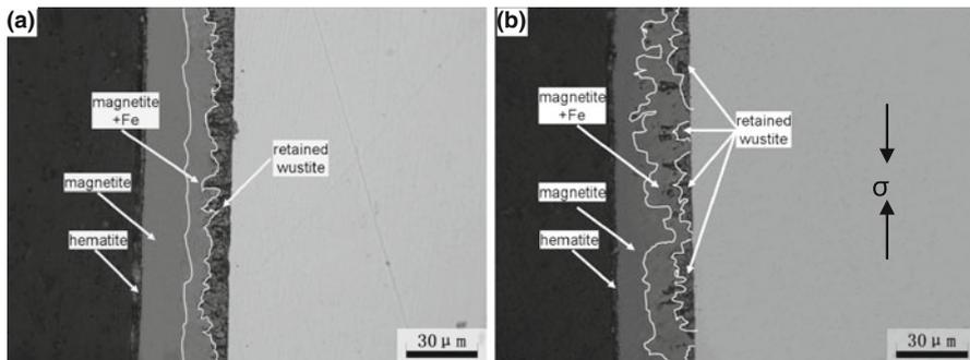
**Fig. 3** Oxide-scale structures developed under a stress of **a** 0 MPa; **b** 10 MPa during furnace cooling at start cooling temperature of 700 °C ( $\rightarrow\sigma\leftarrow$  shows the direction of stress)
