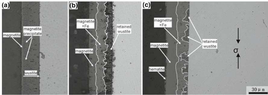
**Fig. 2** Oxide scale structures developed under a stress of **a** 0 MPa; **b** 5 MPa; **c** 15 MPa during air cooling at start cooling temperature of 700 °C ( $\rightarrow\sigma\leftarrow$  shows the direction of stress)
