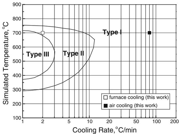
**Fig. 4** Scale type versus simulated coiling temperature and strip-cooling rate [7, 8]
