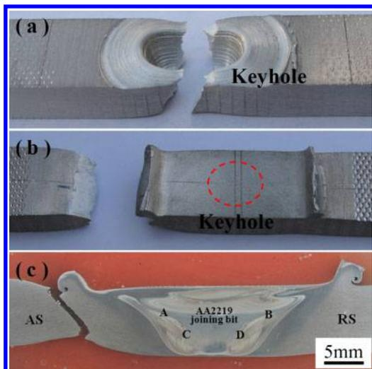
a view of failed keyhole; b view of failed FFSW joint; c cross-section of failed FFSW joint
