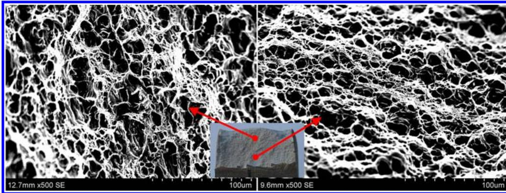
10 Microimaging of FFSW joint tensile fractured appearance
