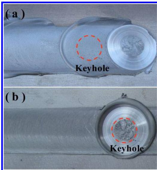
2 Top view of FFSW joints with different processes
