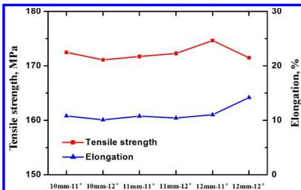
9 Tensile strengths and elongations of FFSW joints
