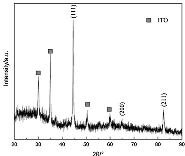
**Fig. 1.** X-ray diffraction pattern of 3D ordered macroporous FeNi alloy thin film electrodeposited on the ITO substrate after the removal of the template.
