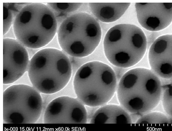
**Fig. 2.** High resolution image of 3D ordered macroporous FeNi alloy film deposited.
