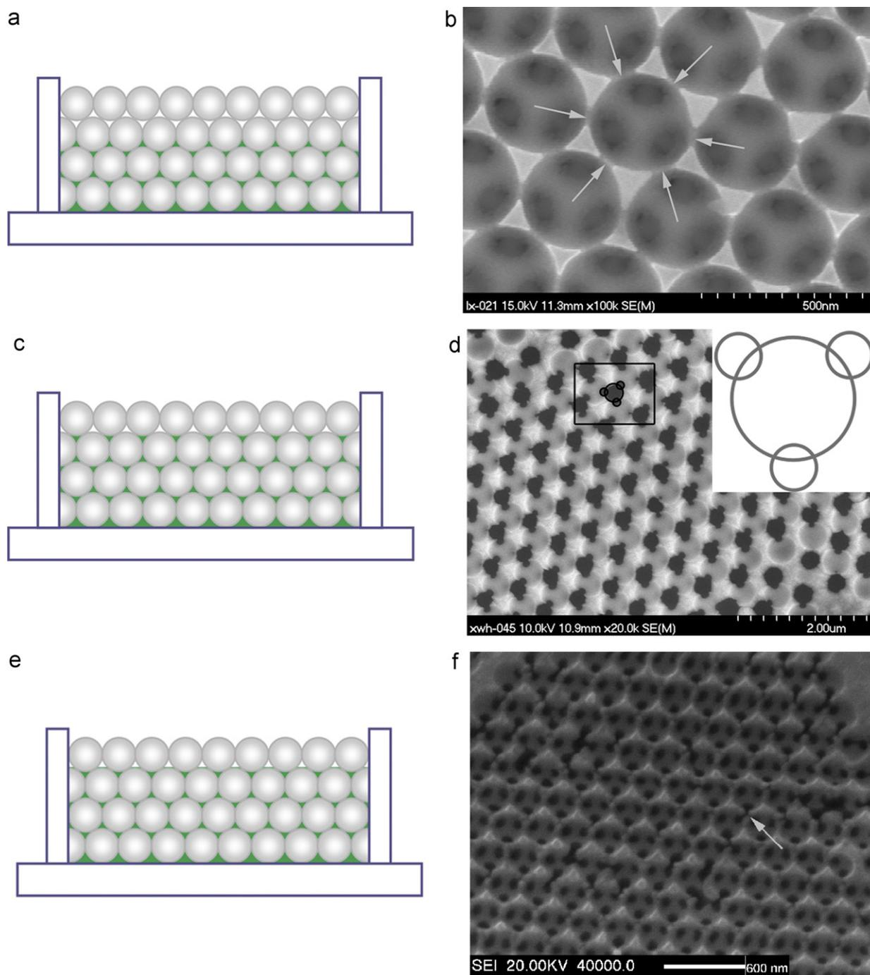
**Fig. 4.** Models of side view (perpendicular to (1 1 1) plane) of the inverse opals and the corresponding SEM images toward (1 1 1) plane at typical film thicknesses.
