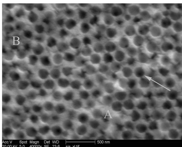
Fig. 5. The morphology of the disordered macroporous FeNi alloy electrodeposited.
