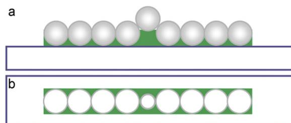
Fig. 6. Schematic illustration of (a) side view and (b) top view of the colloidal template assembled with one sphere arranged at higher position than other spheres of the same layer.
