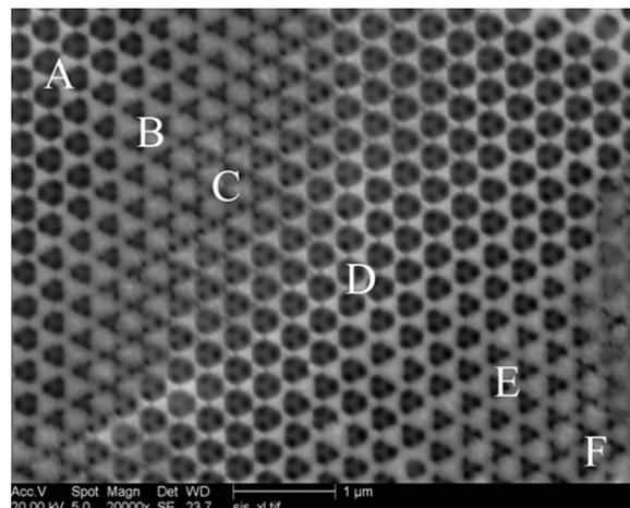
**Fig. 3.** The morphology of a macroporous FeNi film with a gradient thickness electrodeposited through a template assembled from 320 nm diameter spheres.
