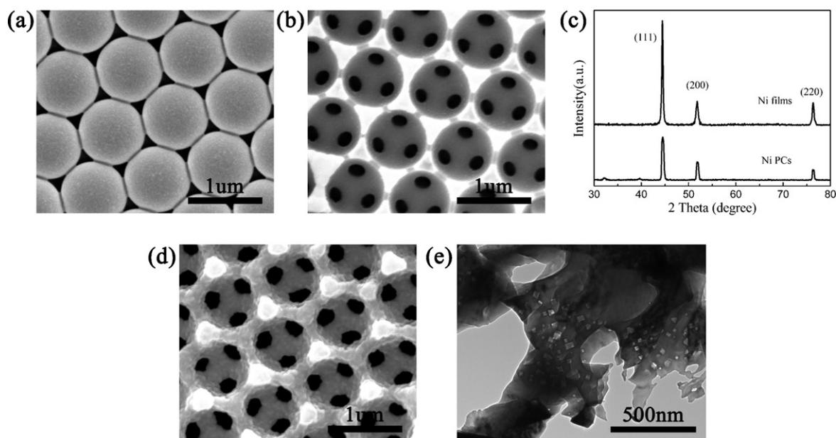
**Fig. 1.** SEM images of (a) PS templates; (b) Ni PCs before annealing; (c) XRD of Ni PCs and pure Ni films; (d) Ni PCs after annealing; and (e) TEM of Ni PCs after annealing.
