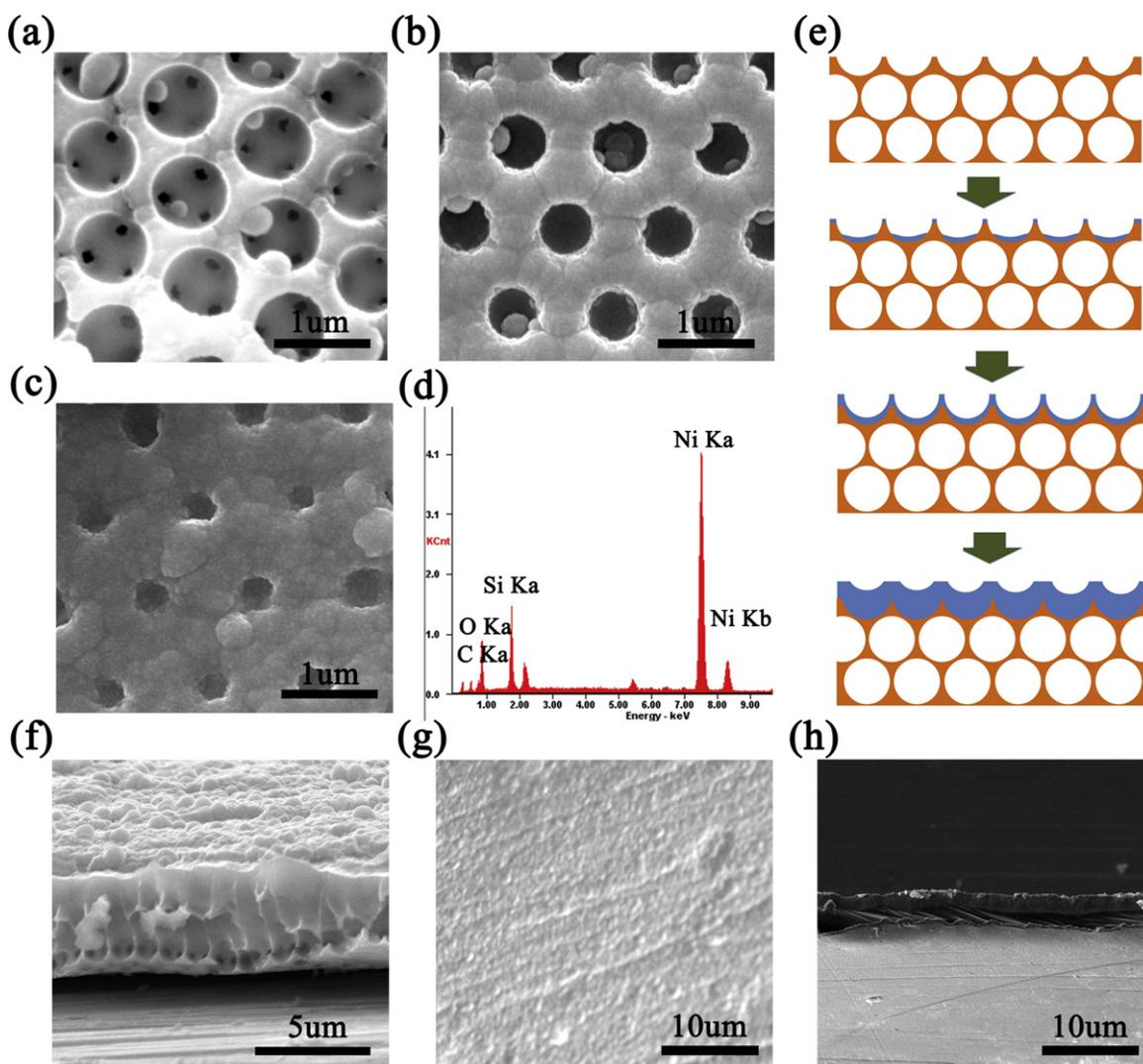
**Fig. 2.** SEM images of Ni PCs/SiC coatings prepared at different deposition time: (a) 1 h; (b) 2 h; (c) 3 h; and (d) the corresponding EDX; (e) the schematic illustration of formation mechanism of Ni PCs/SiC coatings; (f) cross-sectional SEM image of Ni PCs/SiC coatings; (g) and (h) are top-viewed and cross sectional images of SiC coating on pure Ni films.
