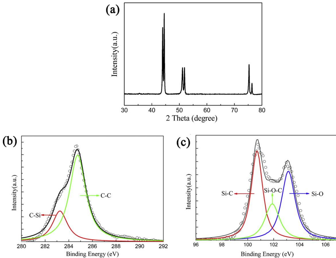
Fig. 3. XRD pattern of (a), XPS spectra of (b), C 1s and (c) Si 2p of Ni PCs/SiC coatings.
