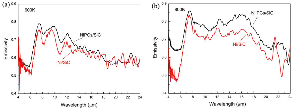
Fig. 4. Spectral emissivity of Ni/SiC and Ni PCs/SiC coatings at (a) 600 K and (b) 800 K.
