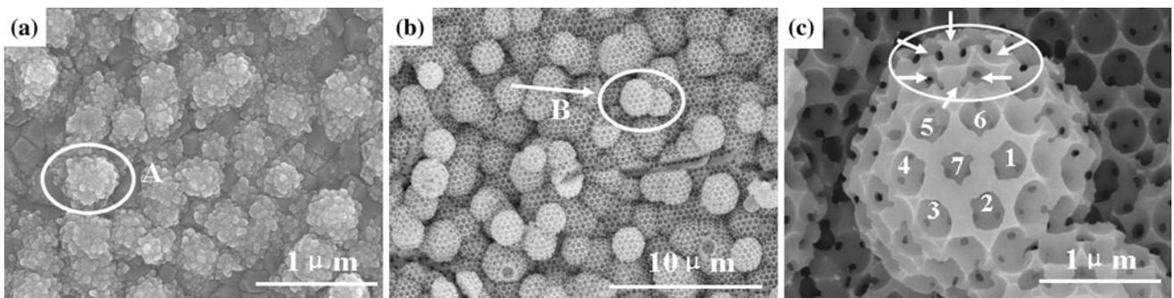
**Fig. 3** **a** The morphonology of  $\text{Cu}_2\text{O}$  film electrodeposited at  $-0.42$  V versus SCE; **b** Template-assistant microporous  $\text{Cu}_2\text{O}$  electrodeposited at  $-0.42$  V versus SCE; **c** The magnification images of the spherical pores
