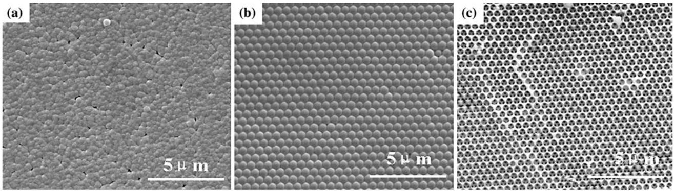
**Fig. 1** SEM images of **a** flat  $\text{Cu}_2\text{O}$  film; **b** well-ordered PS colloidal crystal templates; **c** 3D ordered macroporous  $\text{Cu}_2\text{O}$  structure
