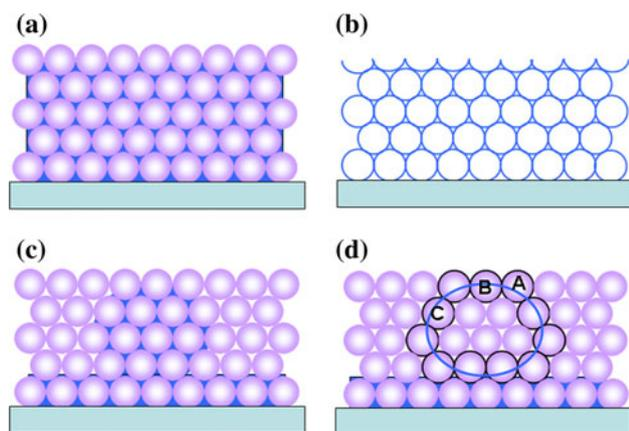
**Fig. 4** Schematic illustration of infiltrating process (*side view*, perpendicular to (1 1 1) plane) based on PS colloidal crystal
