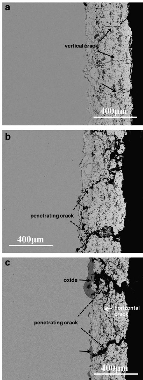
Fig. 4. The cross-sectional morphologies of nanostructured TBCs after (a) 50-cycle, (b) 60-cycle, (c) 150-cycle thermal shock tests.
