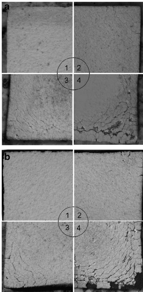
**Fig. 2.** Cracks evolution after thermal shock tests (a) microstructured YSZ; (b) nanostructured YSZ (a<sub>1</sub>) 10 cycles; (a<sub>2</sub>) 30 cycles; (a<sub>3</sub>) 50 cycles; (a<sub>4</sub>) 60 cycles; (b<sub>1</sub>) 10 cycles; (b<sub>2</sub>) 50 cycles; (b<sub>3</sub>) 60 cycles; (b<sub>4</sub>) 150 cycles.
