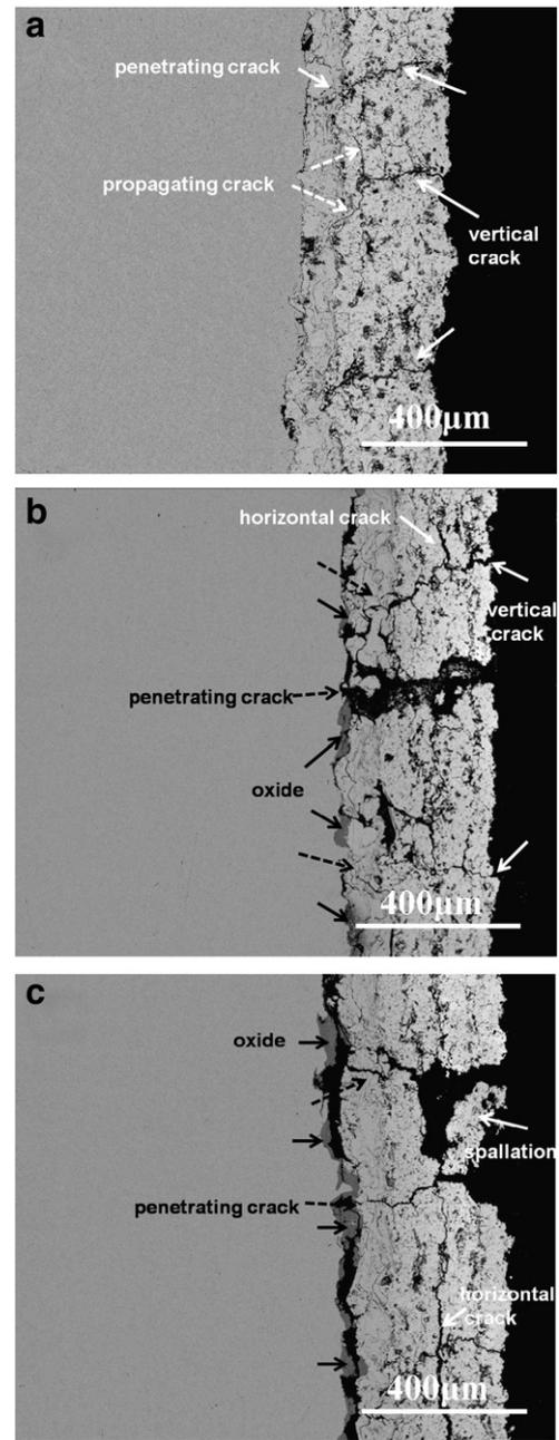
**Fig. 3.** The cross-sectional morphologies of microstructured TBCs after (a) 30-cycle, (b) 50-cycle, (c) 60-cycle thermal shock tests.
