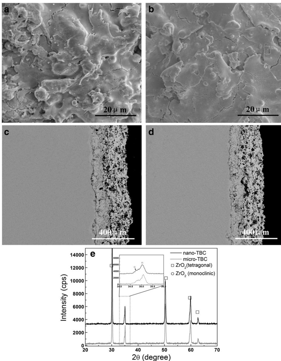
Fig. 1. The surface, cross-sectional morphologies of as-sprayed (a and c) microstructured and (b and d) nanostructured TBCs, and (e) the phase compositions.
